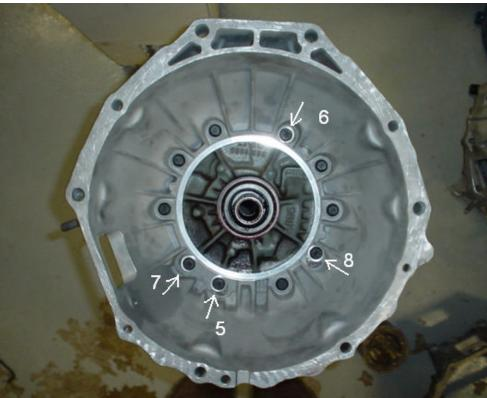
Figure 7 – VG30 bellhousing installed, long bolt torque sequence
