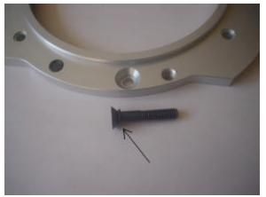
**Figure 3** – front o-ring installed on tapered bolt
