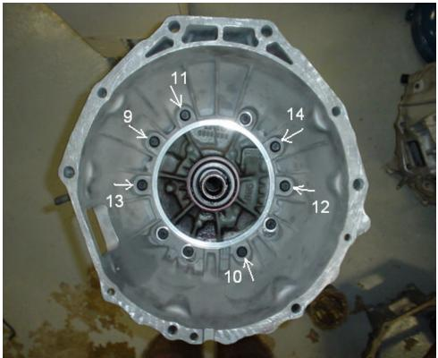
Figure 8 – Short bolt torque sequence
