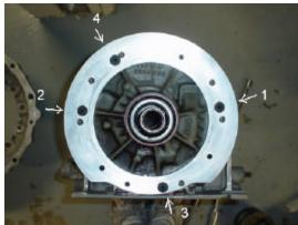
Figure 6 – Adapter installed, torque sequence
